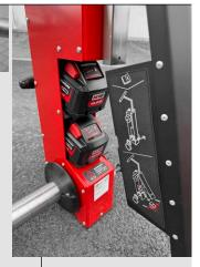
**Electric motor powered** by 18 V batteries
